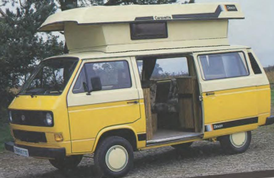
An ingeniously designed elevating roof with fully insulated rigid panels distinguishes the Caravette.
