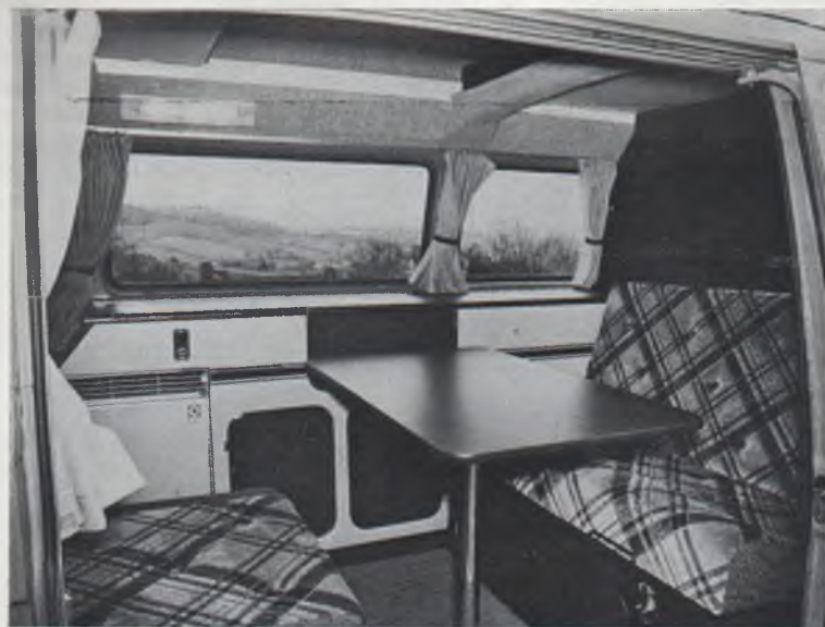
Moonraker interior. The seat nearest the camera is removable and a swing-out frame on the far side provides an additional seat when needed. The double seat folds very easily to provide the double bed. Sink is in the cabinet above the 'fridge (switches control 'fridge operation and pump for tap), cooker is behind darker section. Wardrobe can be seen behind double seat.
