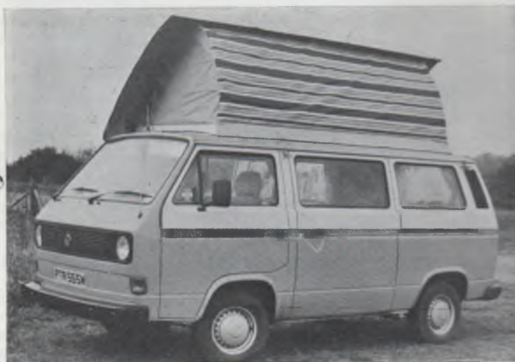
The Moonraker with roof elevated. Gas struts make raising it an easy job.
